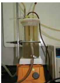
The CDC biofilm reactor, developed by the Centers for Disease Control and Prevention (CDC) in 2002
